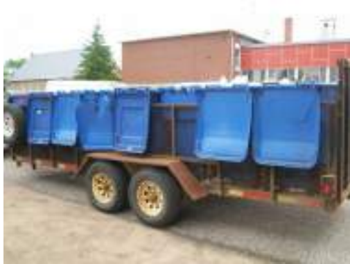
The collection trailer and material totes, which are loaded from the top.
